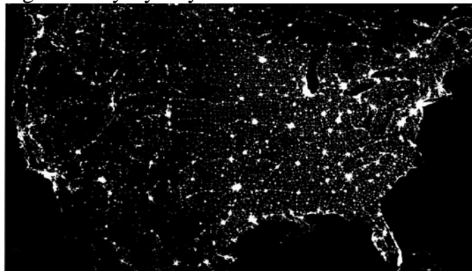
Location: United States Data gathered by: U.S. Defense Meteorological Satellite Program (DMSP) spacecraft Instrument: Operational Linescan System (OLS) Uses of information: This image of nighttime city lights was produced with data gathered during 186 orbits of the DMSP F-12 satellite and 50 orbits of the F-10 satellite from October 1994 through March 1995. The OLS is able to detect faint sources of visible and near-infrared surface emissions, including city lights, gas flares and fires. To filter out nonstable lights, such as fires and lightning, researchers at the U.S. National Atmospheric and Oceanic Administration determined the number of times a light was detected during a cloud-free observation. Thus in this image, most of the detected features are lights from cities and towns, although oil platforms are visible in the Gulf of Mexico. City-light maps, which are indicators of human population distribution, can be useful in studies of human impact on the environment, according to the researchers.
